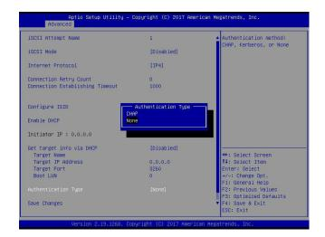
**Note:** Challenge handshake authentication protocol (CHAP) is a protocol used to verify the identity of the peer of a connection.
