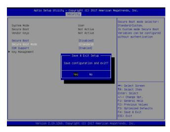
Step 3. Press <Del> during system boot to enter the BIOS Setup utility. Navigate to the Security tab and enter the Secure Boot menu. Set CSM Support to Disabled.
