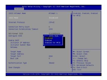
**Note:** Enabling the feature, iSCSI Mode, is required for iSCSI configuration.
