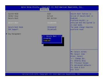
For the changes to take effect, press <F4> to save the settings and exit the BIOS Setup utility. Press <Del> during system boot to enter the BIOS Setup utility. Navigate to the Security tab and enter the Secure Boot menu. The following screen will appear.
