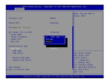
**Note 1:** If one way (unidirectional) CHAP authentication is performed, the iSCSI target authenticates the iSCSI initiator.
