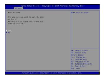
**Note:** A spare disk is used for automatic RAID volume rebuilds when status of failed, missing, or at risk is detected on the array disk. For a RAID0 volume, only status of at risk will trigger automatic RAID volume rebuilds.
