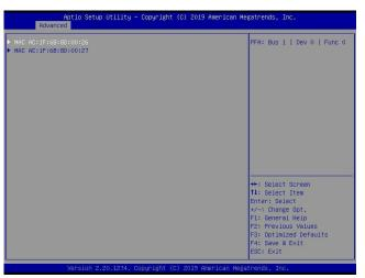
Press <Enter> and the following screen will appear. Use the arrow keys to select the desired media access control address (MAC address), network interface card (NIC) port.
