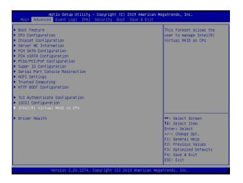
14. Use the arrow keys to select Intel(R) Virtual RAID on CPU and press <Enter> to access the menu items. The following screen will appear showing that the feature "**All Intel VMD Controllers**" has become available.
