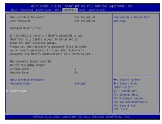
Use the arrow keys to select Secure Boot and press <Enter> to access the menu items. The following screen will appear.
