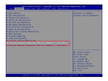
Press <Enter> and the following screen will appear. It displays the detailed information for the selected onboard LAN device.
