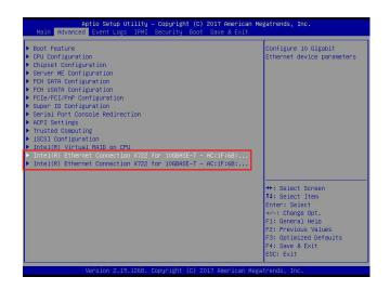
Use the arrow keys to select the desired onboard LAN device as shown below.
