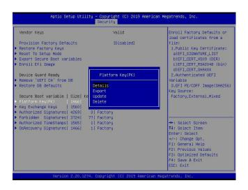
Details: Use the arrow keys to select Details and press <Enter>. It displays detailed information of PK as shown below.
