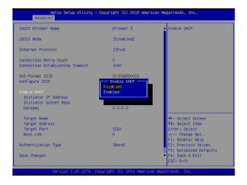
**Note:** Set the feature, Enable DHCP, to Disabled if you would like to specify the iSCSI initiator IP address/subnet mask/gateway.
