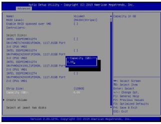
Enter the desired RAID capacity (in GB) in the pop-up menu to set the capacity for your RAID volume.
