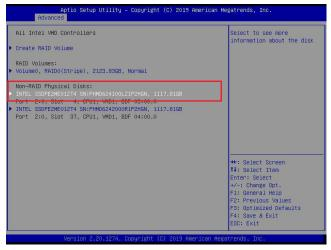
After a NVMe device is selected, press <Enter> and the following screen will appear. Select **Mark as Spare** and press <Enter> to mark the selected device as a spare device.
