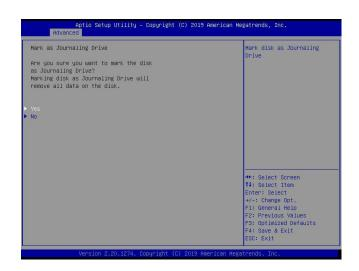
**Note:** RAID Write Hole (RWH) is a condition associated with a power/drive-failure/crash while writing to a RAID5 volume. The use of journaling drive that contains partial parity logging (PPL) can reduce the potential data loss. Refer to the following illustration for the use of journaling drive.
