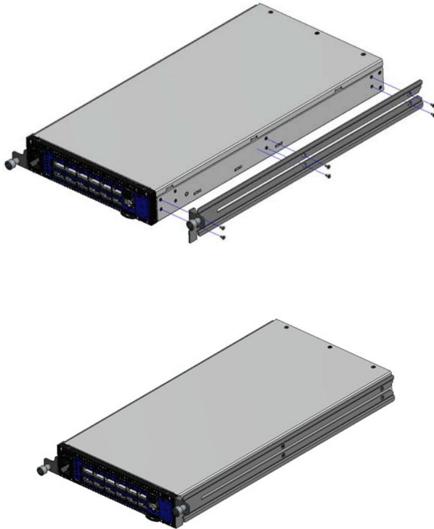
Figure 12: Screw on the System Mounted Rails
