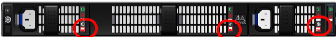
Figure 2: Air Flow Direction Marking - Connector Side Inlet to Power Side Outlet
