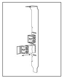
2. The adapter ships with one bracket installed and another size bracket in the shipping container. If the installed bracket works as is, go on to Step 3.
