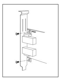
3. Insert the adapter into the desired empty PCIe bus slot. Press firmly until the adapter is seated.
